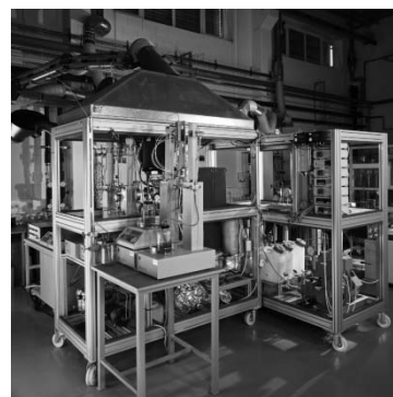
Figure 2: Continuous flow reactor system at Fraunhofer ICT
