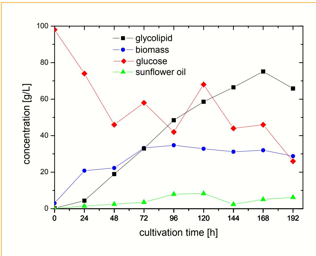
**5 L fermentation with sunflower oil and glucose feeding using integrated ultrasound separation:**
