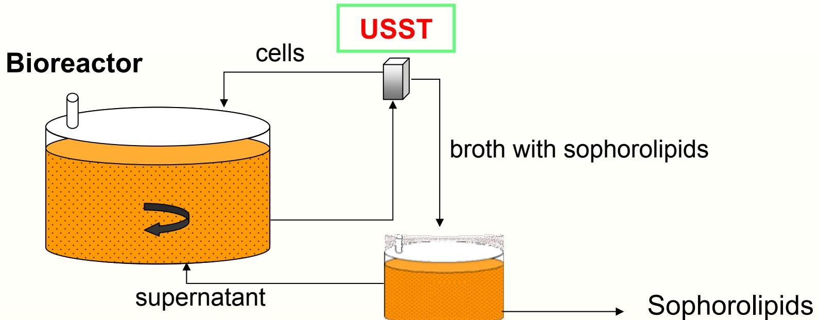
**Small reactor:** settling vessel for sophorolipids
